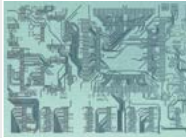
Direct exposure of resists (ultrafine conductor production)
