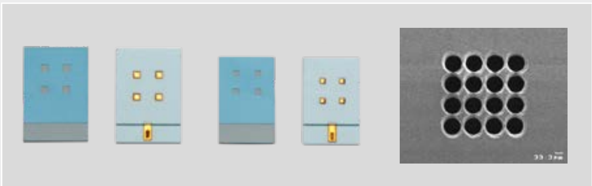
The UV laser cuts, engravings and drills mechanically sensitive substrates, such as LTCC components.
