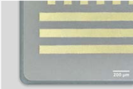
Cutting GaN and the geometrically accurate ablation of μm thick copper/gold coatings
