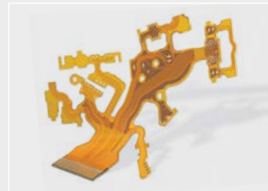
Cutting populated and unpopulated materials – even into complex shapes: ceramic, polyimide, and FR4
