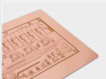
Laser-structured FR4 boards feature an extremely good match between layout and actual geometry
