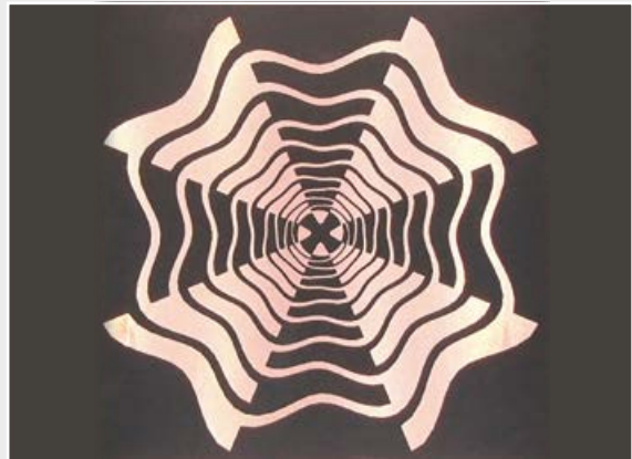
Rogers RO 5880 Antenna (works also on RO 3003, RO 4003)
