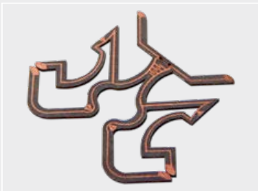
Structured and cut-out example of an RF circuit on an RO 5880 material
